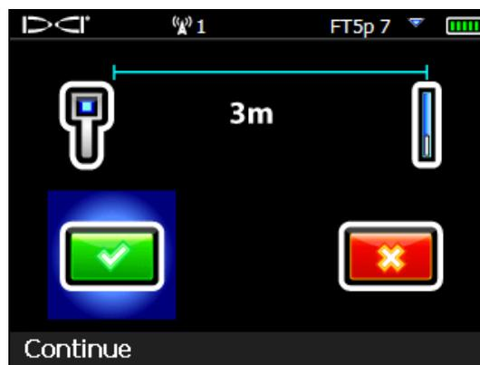
6. Do not move the receiver. A successful calibration yields a check mark
