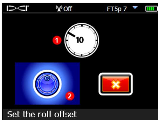
1. Transmitter's true roll position with housing at 12:00
