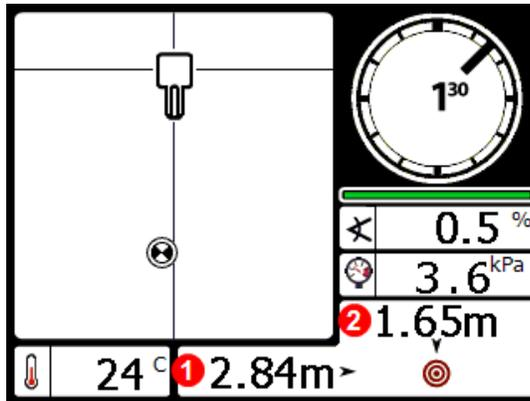
1. Horizontal distance from transmitter to receiver
