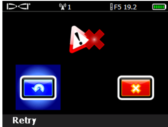
2-Point Calibration Failure Screen
