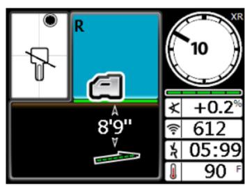
3. When the roll and pitch data display is steady, and before the reading counter reaches 99 and restarts, note the data and release the trigger.
