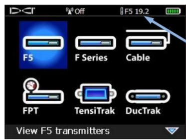
Current transmitter type (F5) and frequency (19.2) are shown at the top
