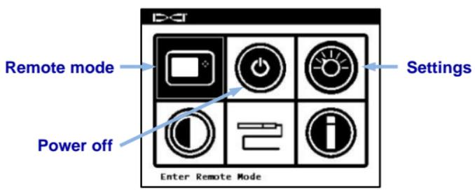
Use the arrow buttons to highlight menu options and **Execute** to select. Use **Remote Mode** during drilling.
