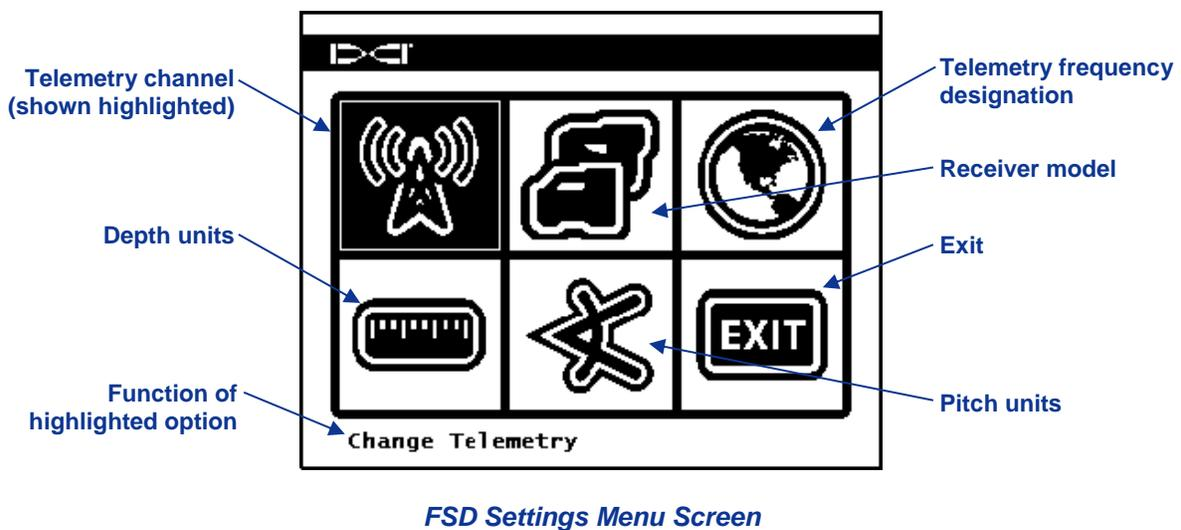
The table below shows the menu options as they appear on the display with descriptions of their uses. Any changes that are made to the settings will be saved when the FSD unit is turned off. DCI recommends that you program the FSD settings to match the settings on your receiver.
