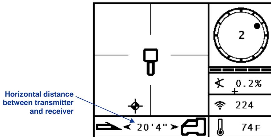
*Receiver Screen with Target Depth Programmed*
