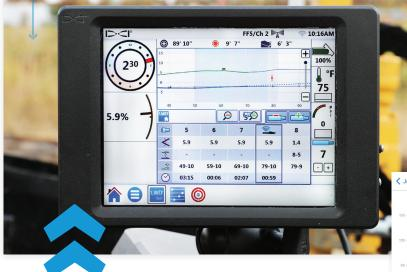
Full bore plans can then be transferred to an **AURORA** remote display where drillers can see real-time, rod-by-rod progress and projections.
