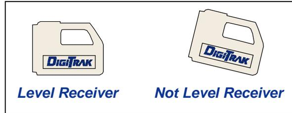
You can track the transmitter by holding the receiver while facing the drill or while facing away from the drill (see figures below). Either way, the information on the receiver display will be the same when at the same location. For an accurate depth reading, you must hold the receiver level and have it aligned with and directly above the transmitter.
