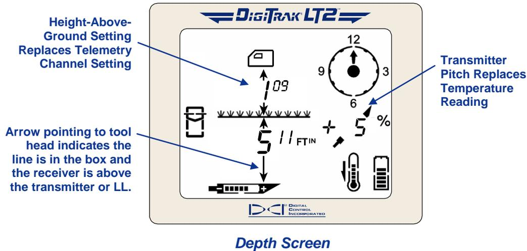
**NOTE:** The arrow that appears below the depth measurement and that points to the transmitter also appears on the remote display when the line is in the box.
