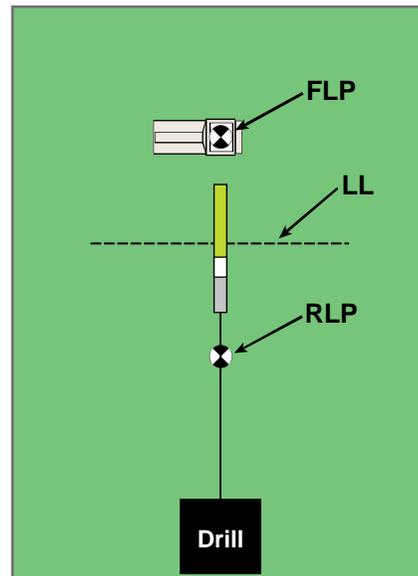
*Turn Receiver 90° and Move Back and Forth to Center Target in Box at FLP*
