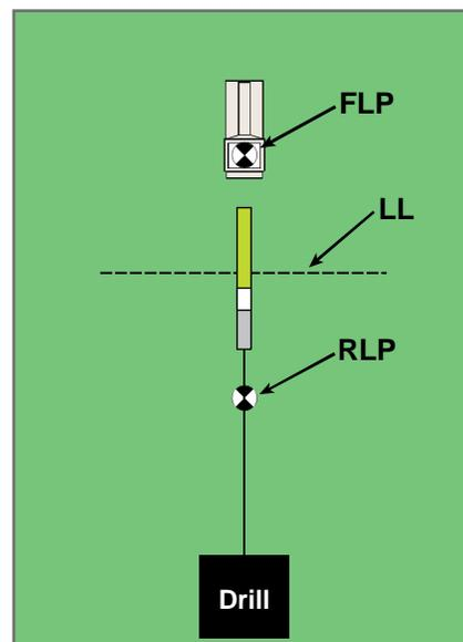
4. Turn the receiver 90° from the transmitter heading while holding the receiver steady and level, and again center the target in the box by moving the receiver forward or backward as needed. This is the FLP, which is where the transmitter will end up if it does not get a steering command.
