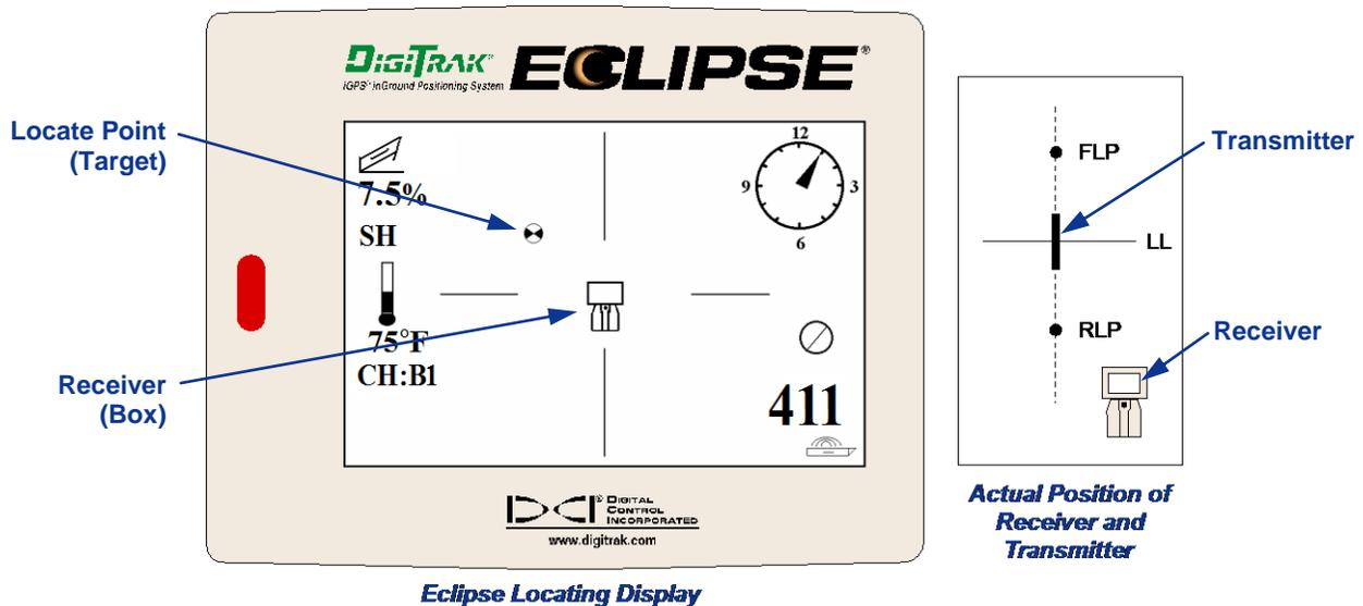
2. Position the receiver until you get the target in the box as shown below. You are now standing with the receiver positioned over the RLP.
