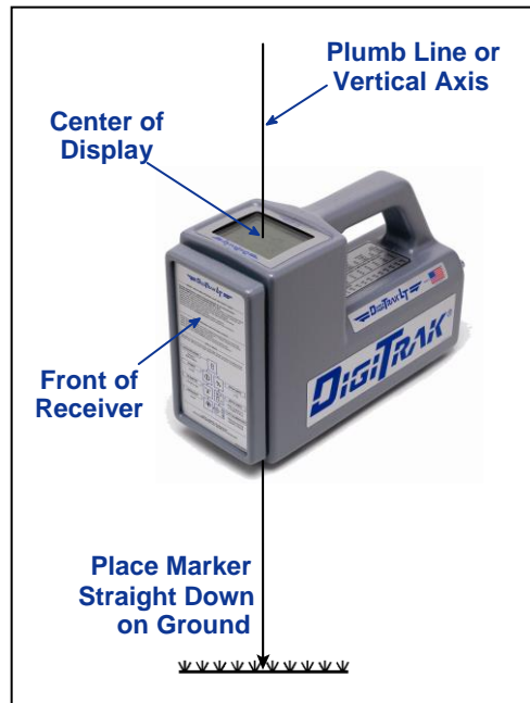
Plumb Line for Marking Locate Points
