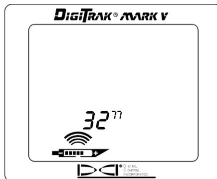
**Receiver Frequency Display After Releasing Held Trigger**
