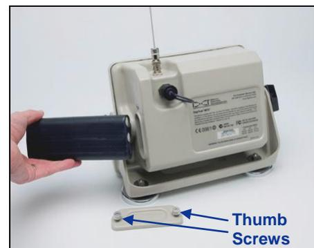
**Inserting Battery into MFD Remote**
