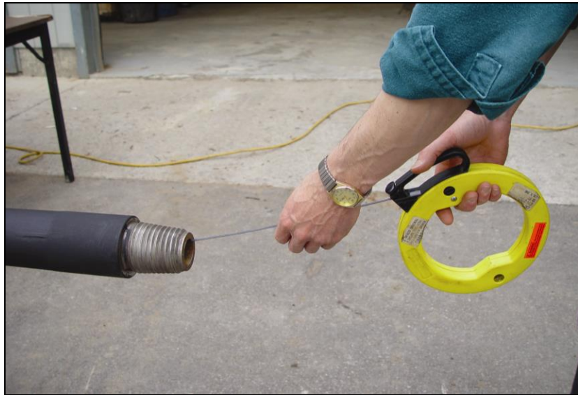
Pushing Fish Tape into Rod from Pin End to Box End
