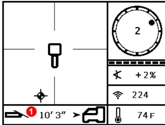
1. Horizontal distance from transmitter to receiver
