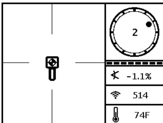
**Receiver Locate Screen at RLP**
