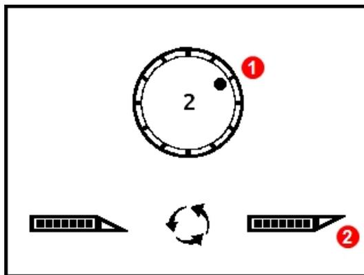
1. **Transmitter's true roll position with housing at 12:00**
