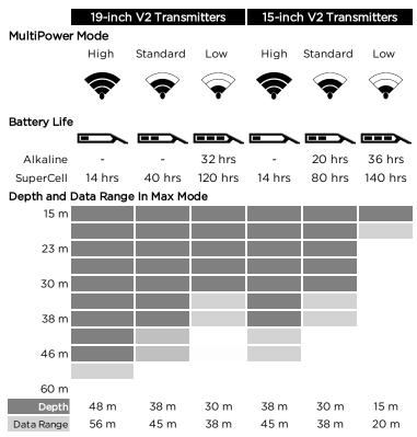
The battery types listed are the only types recommended for that model and size. DCI does not recommend using other battery types.
