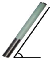
Hold the Tx at the same ( $\pm 2$ ) general clock position (CP) for this whole procedure. Hold Tx powered on at level ( $0 \pm 10^\circ$ ) for at least five secs. Tilt Tx up at approx.  $+65^\circ$  (almost vertical) for 10–18 secs., then return to level for 10–18 secs. When the Tx changes bands, data disappears from the locator.
